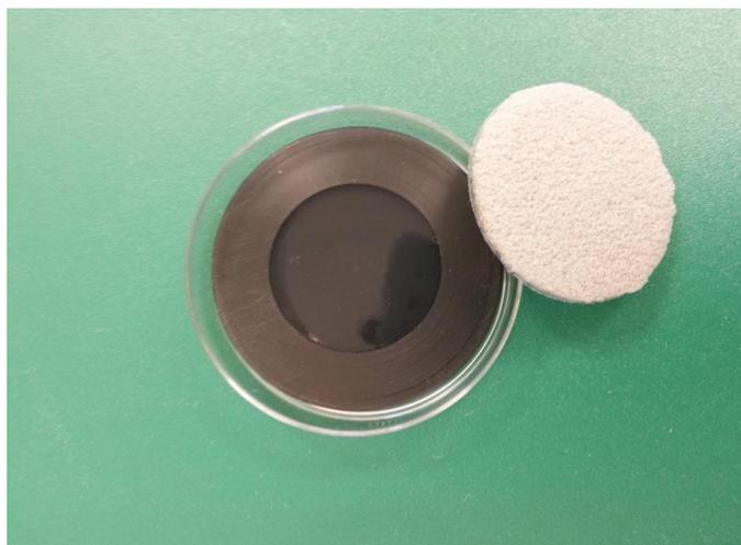
Figure 5 Acceptor compartment consisting of agar in POM ring equipped with bottom and piece of Mepilex® Ag dressing.
