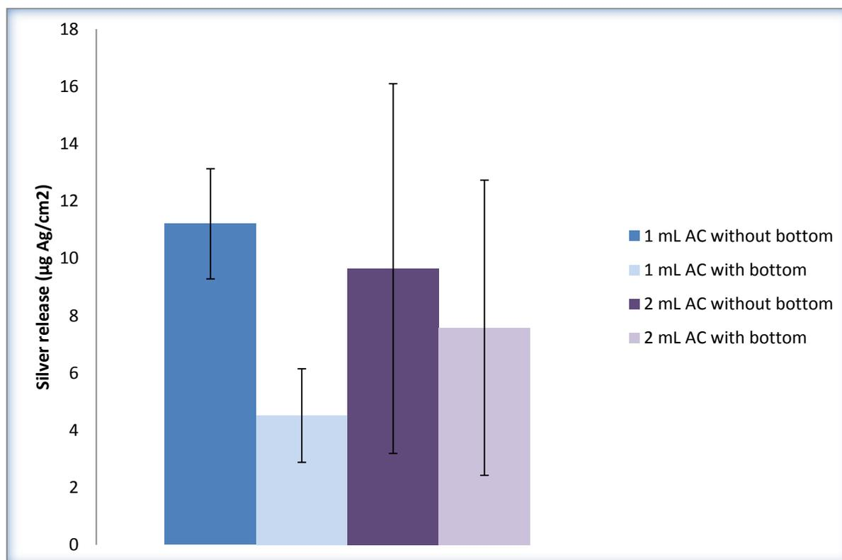
**Figure 9** Silver release in µg Ag/cm<sup>2</sup> measured from Mepilex® Ag on agar pre-wetted with SWF to 100% saturation. Error bars represent standard deviation. n = 4.
