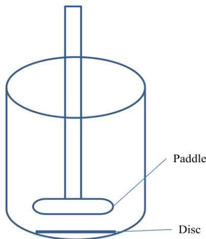
**Figure 2 Schematic illustration of Paddle over disc.**
