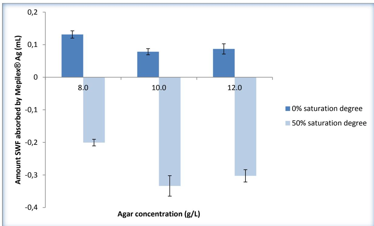
**Figure 8** Amount SWF absorbed by Mepilex® Ag at different agar compositions. Error bars represent standard deviation. n=3
