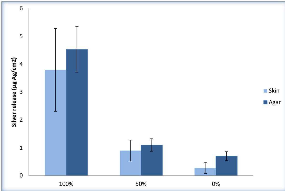
Figure 10 Silver release from AC consisting of skin and agar at different degree of moisture saturation with SWF. Error bars represent standard deviation. n = 4 for agar and 3 for skin.
