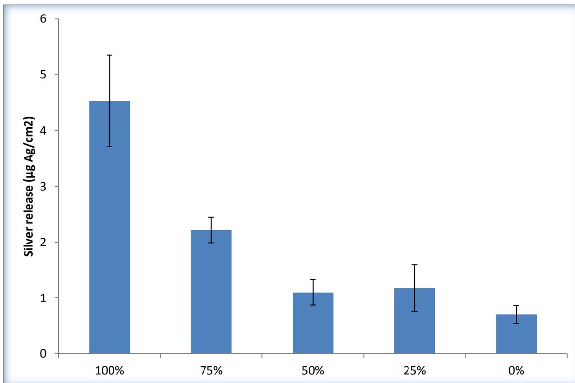
**Figure 12 Silver release measurements at different degree of moisture saturation with SWF. Experiment performed on 1 mL AC with ring equipped with bottom. Error bars represent standard deviation. n= 4.**
