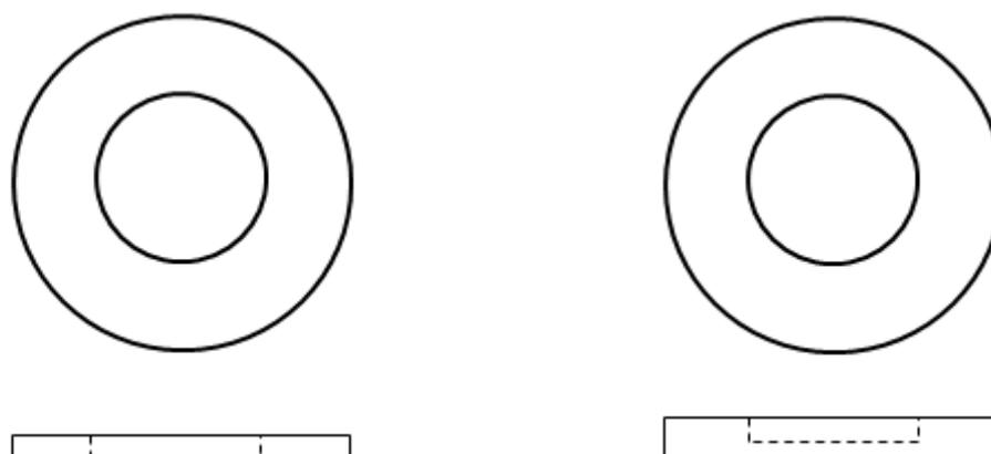
Figure 4 Schematic illustration of 1 mL POM ring without bottom (left illustration) and with bottom (right illustration).
