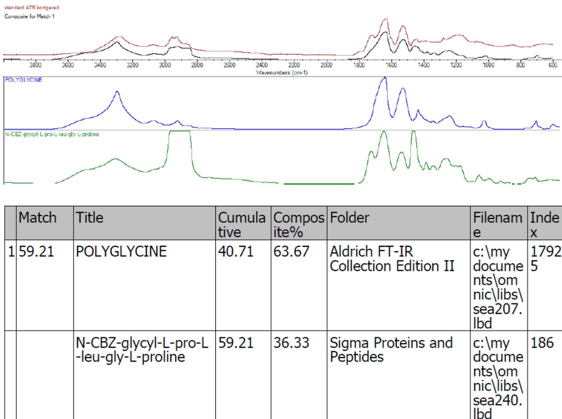
**Figure 17** A multi-component search using FTIR for analysis of the precipitation. This is compared to a protein database.
