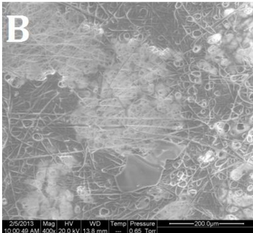
Figure 15 SEM picture from analysis of precipitation on glass fiber filter. Picture A obtained from backscattered electrons, picture B obtained from secondary electrons.
