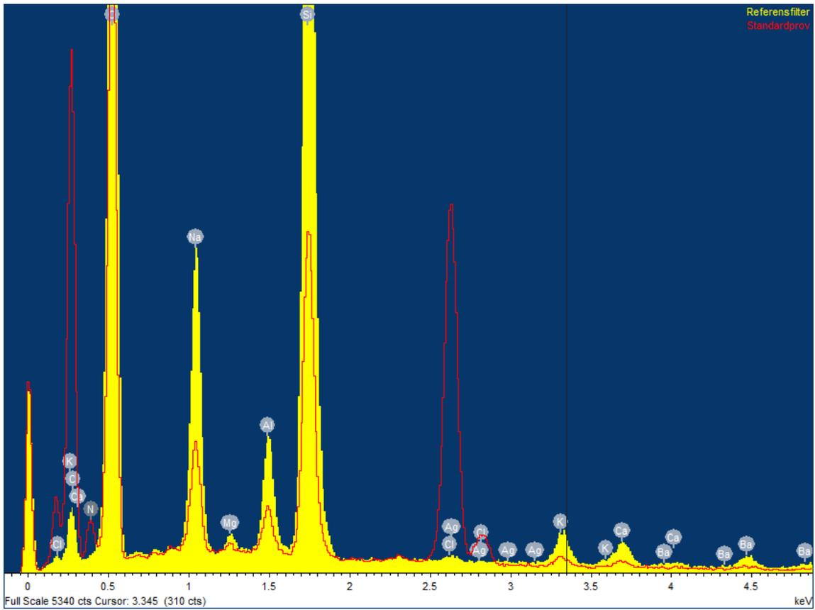
Figure 14 SEM analysis performed on the precipitation obtained from digestion of acceptor compartment. The red curve represents the precipitate while the yellow graph represents a reference filter paper.
