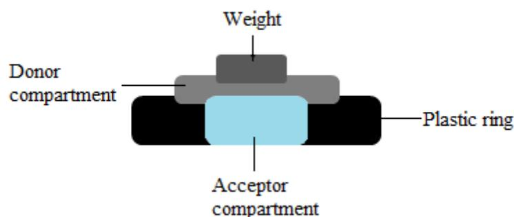
Figure 6 Schematic illustration of the set-up of the plastic ring (without bottom) with acceptor compartment, dressing and weight.
