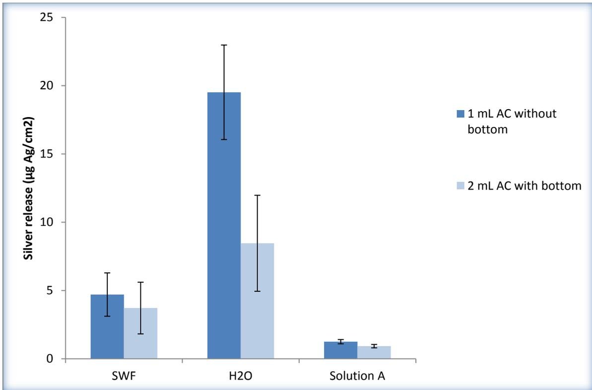
**Figure 11 Silver release dependent on type of fluid used for pre-wetting. Experiment performed on 1 mL AC without bottom and 2 mL AC with bottom with agar as gelling agent. Error bars represent standard deviation. n= 4.**
